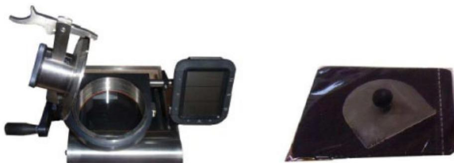
In order to complete the Cobb test you will also need blotting papers from 200 to 250g/m<sup>2</sup> and an analytic scale with an accuracy of 0.001g.
