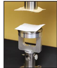
▲ ZDT Tester measures the internal bond strength of paperboard.
